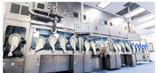
ChargePoint AseptiSafe Bio Valve® Integrated into Evonik's Isolator Process
